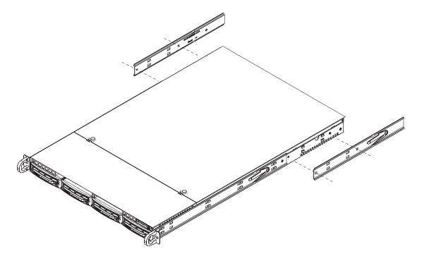
Figure 2-2. Installing the Rack Rails
